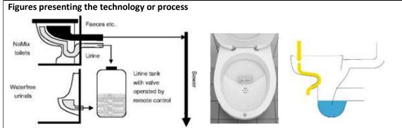
*Figure 1. Principles of urine source separation technology and example of two toilets with and without (type Laufen: SAVE) a separate bowl for urine collection.*
