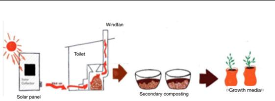
Figure 3. Principle of the solar assisted toilet to be used in SiEUGreen case Århus. The solar panel is attached to the south side of the toilet and provides both warm air and electricity to power a fan.
