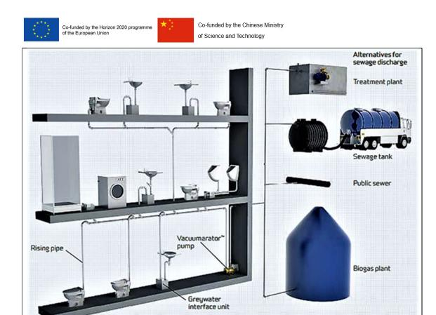
Figure 1. System design example with various discharge options. (Source: JETSGROUP, 2013)
