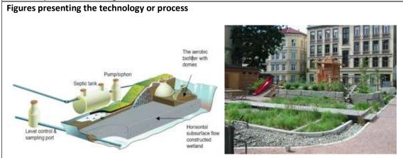
Figure 1. Filterbed system with integrated aerobic biofilter for greywater treatment (Jenssen and Vråle, 2003) and a biofilter combined with constructed wetlands for greywater treatment in Oslo
